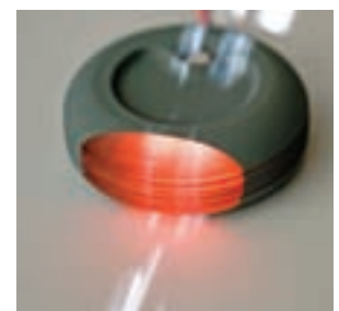
A landing gear control knob assembly with red NVIS lighting
