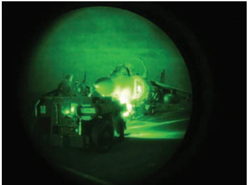
A Harrier aircraft with incompatible lights around it in an NVG shot
